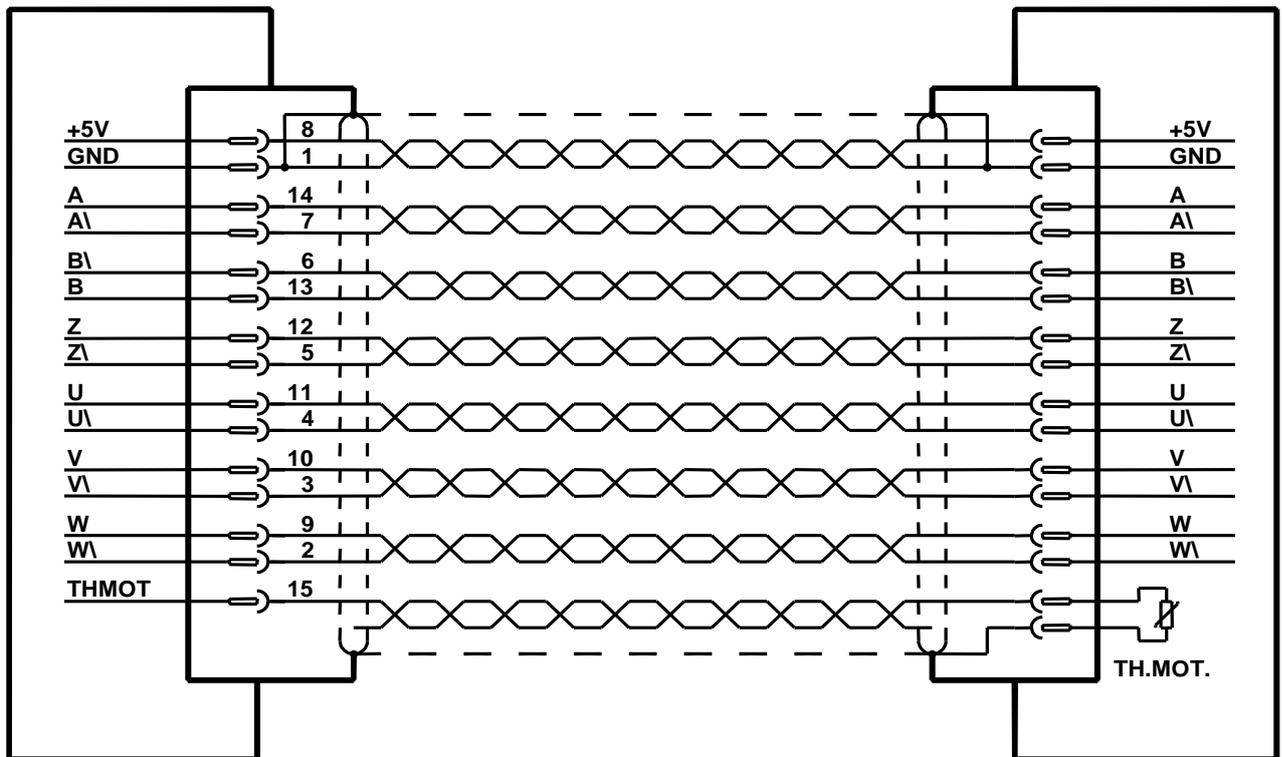
A, A/, B, B/, Z, Z/, U, U/, V, V/, W, W/, 5V, GND and Th.mot. To work properly and with respect of the trigonometric sense of rotation, B and B/ must be crossed.
